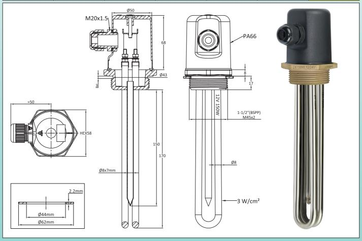
Main application: direct use of low voltage electricity produced by wind turbines or photovoltaic solar panels, for heating liquids, domestic hot water circuits, hot water tanks. These immersion heaters make it possible to use the surplus energy produced, and not used by domestic lighting needs or small electrical appliances. They can also be used in addition to domestic hot water tanks, limiting the need for electricity from the distribution network.
